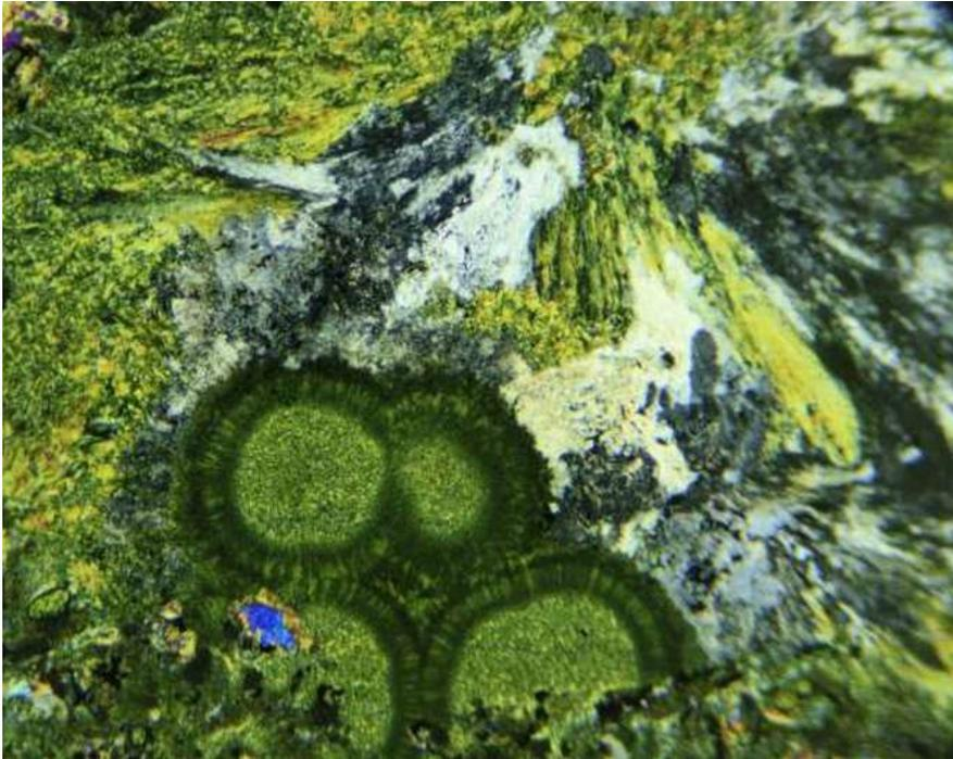
Figure 1: Basalt 40x, (4x obj. + 10x eyepiece). Labomed CxL microscope with simple polarizing kit. Canon 5D MkII, ISO 400, 1/3 sec. The camera sees the optical path as an  $f$  0.0 50mm lens.
