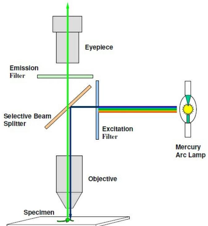
Figure 1: Schematic of typical fluorescence microscope.
