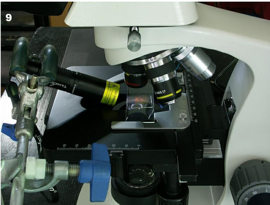
**Figure 9:** Using the UV torch to illuminate a specimen of algae under the microscope.
