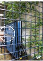
Here, the camera is not well positioned. The rotation axis is just 10 mm behind the entrance pupil. Note the shifts between the background and the verticals of the grid (window frame, flower jars, table-tennis table, etc.).
