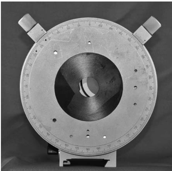
FIGURE 3.7 Rotatable stage for PLM (note 1-degree graduations plus Vernier scale).
