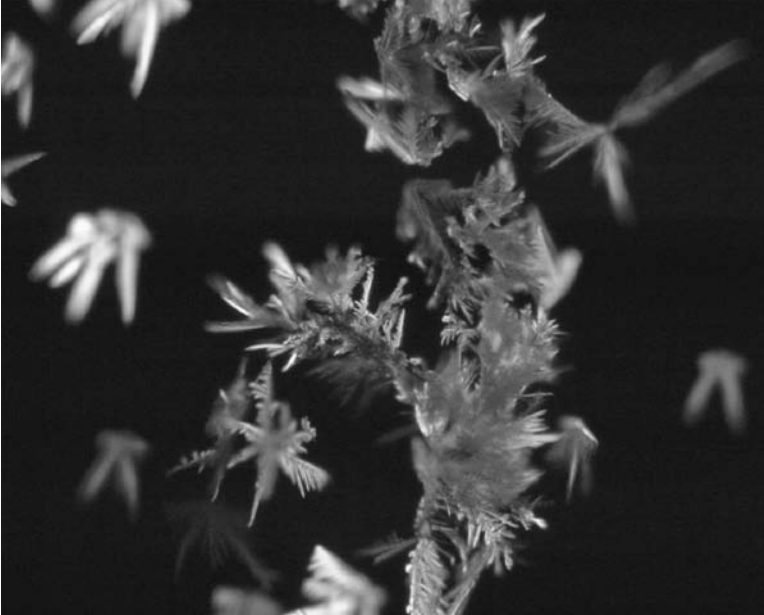
FIGURE 9.4 Crystals formed by gold chloride and cocaine, here created in an agarose gel. This is a useful technique for obtaining images showing crystal growth habits.
