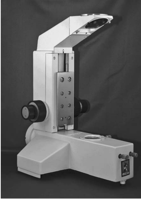
FIGURE 3.1 A microscope stand must be stable, accommodate all attachments, and provide a clear optical pathway.
