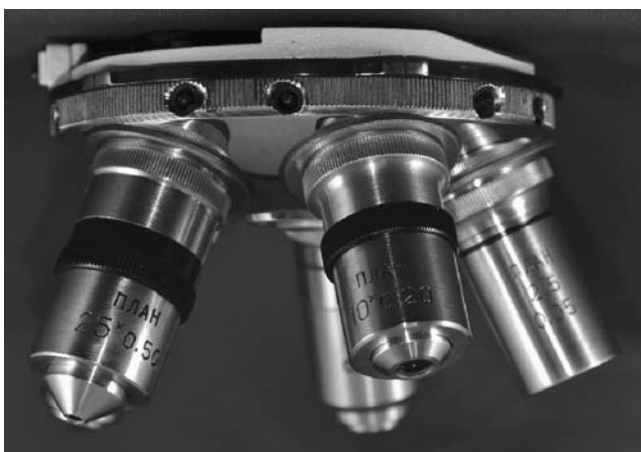
FIGURE 3.3 Nosepiece holding five objectives. Note that adjusting screws allow centering of objective in polarized light microscopy.
