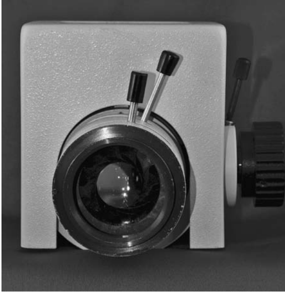
FIGURE 3.10 Lamp holder (see Figure 3.9) inserted into lamp housing (on right). Threading on the lamp holder allows adjustment of the filament on the x axis. The rod just above allows adjustment along the y axis. Looking down the optical axis, one sees two levers. The front lever adjusts the focus of the filament and the second lever adjusts the field diaphragm.
