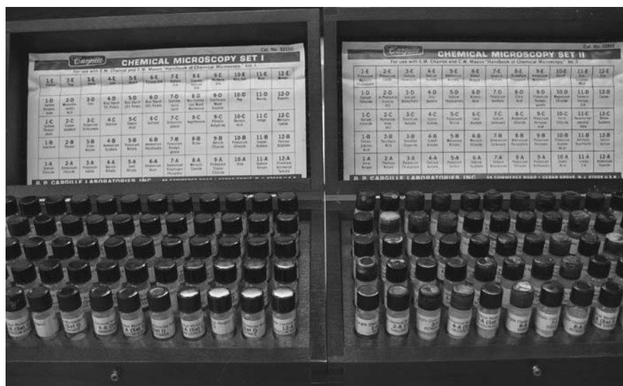
FIGURE 9.3 Chemical microscopy kits. The few milligrams in each reagent bottle will last for years.
