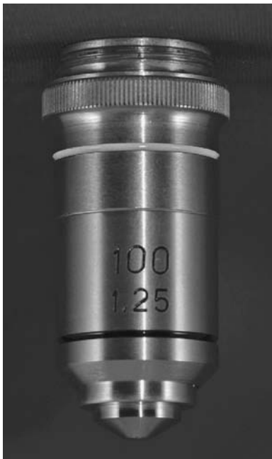
FIGURE 3.2 100× 1.25 NA achromat objective.
