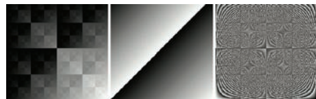
Figure 3.2 Three possible results from draw-values . The draw-values function you've written can be used to create a variety of graphics. Here are examples, from left to right, of bit-and , + , and * .
