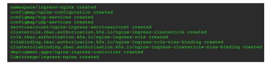
Figure 4.8 - NGINX installation output
