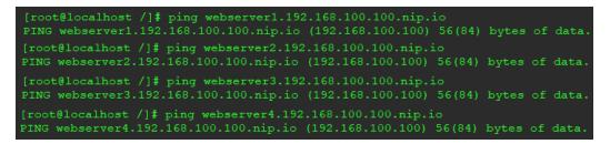
Figure 6.4 - Example name resolution using nip.io
