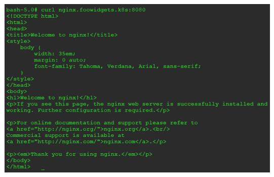
Figure 6.17 - Curl test using the external-dns name
