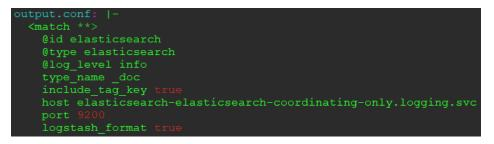
Figure 12.10 - Fluentd output configuration
