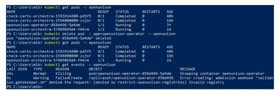
Figure 11.4 – Pod fails to create because of GateKeeper policy
