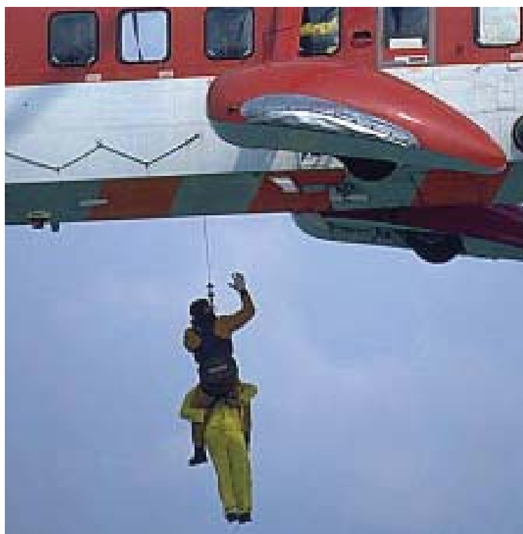
A rescue swimmer and victim are winched aboard a British Coast Guard helicopter. If the victim were to raise his arms he could fall out of the lifting strop. The U.S. Coast Guard swimmers usually put their legs outside of your arms to avoid this possibility.
