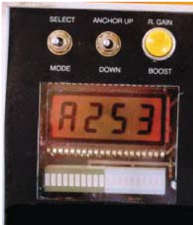
The WH autopilot control head on Beowulf is typical of what we've used on our clients' boats for over 15 years. Note the three manual controls for gain, counter rudder, and yaw (also known as dead band or sea state).
