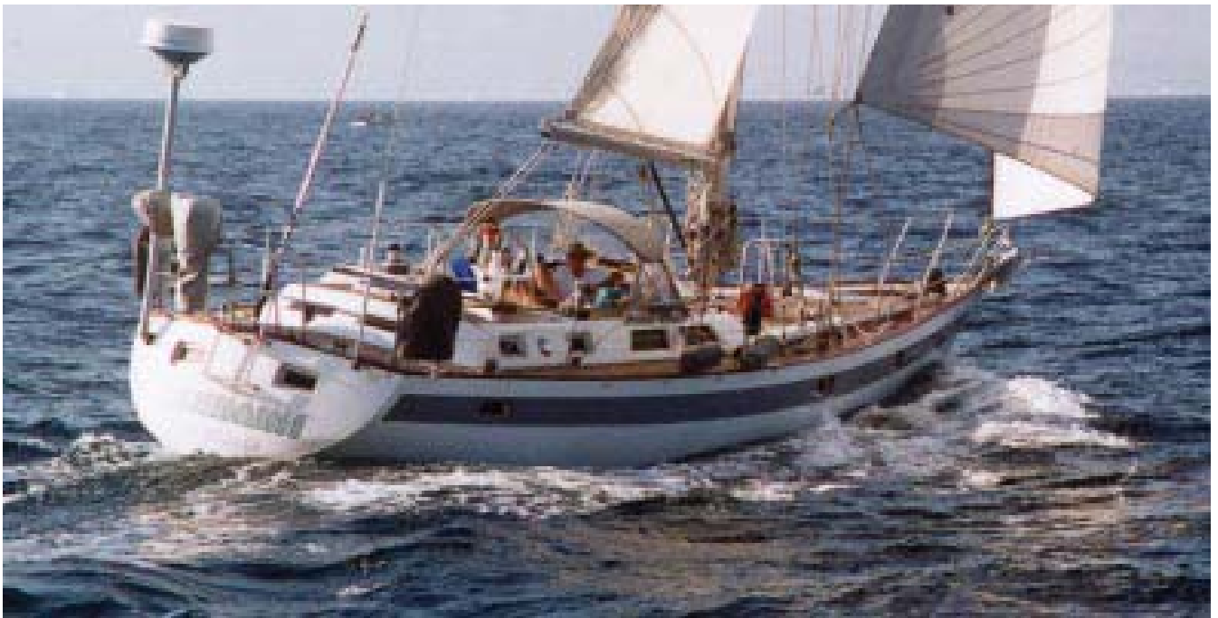
Shakti is 44 feet 7 inches (13.7m) long, 39 feet (12m) at the waterline, with a beam of 13 feet (4m) and draft of 6 feet 6 inches (2m). As cruising boats go, she's relatively quick.
