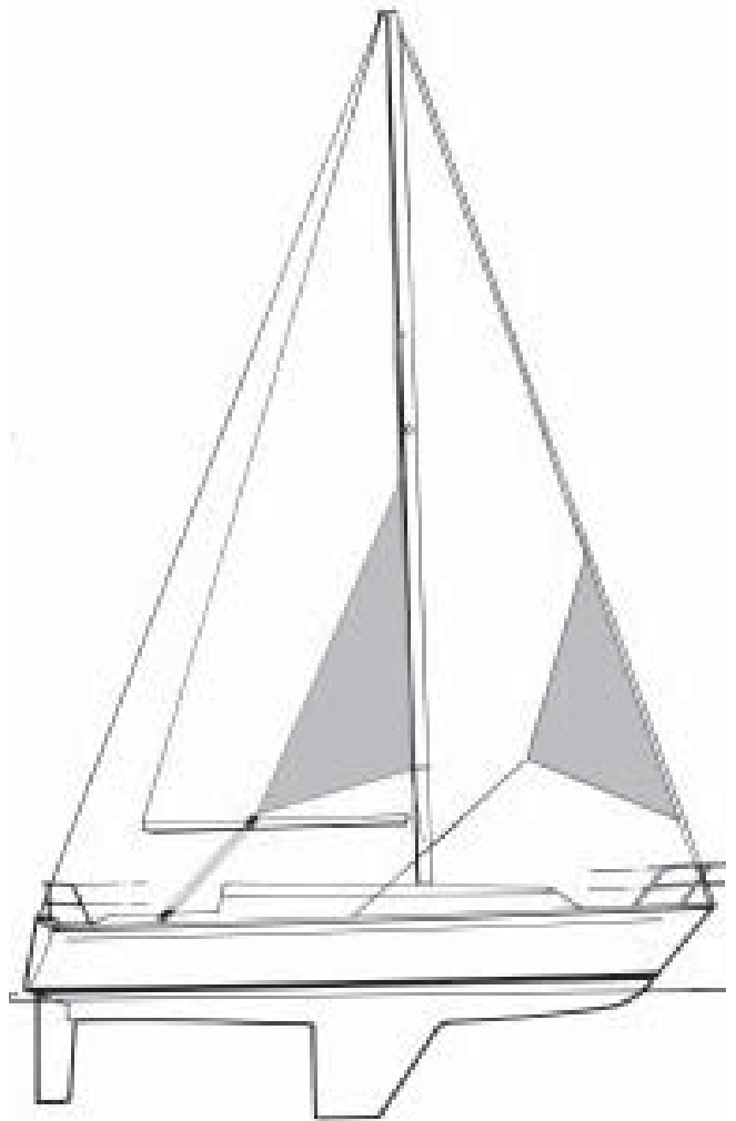
The proportions shown here are for storm-force-and-above wind strength. These sails are smaller in scale than the norm based on ORC regulations.
