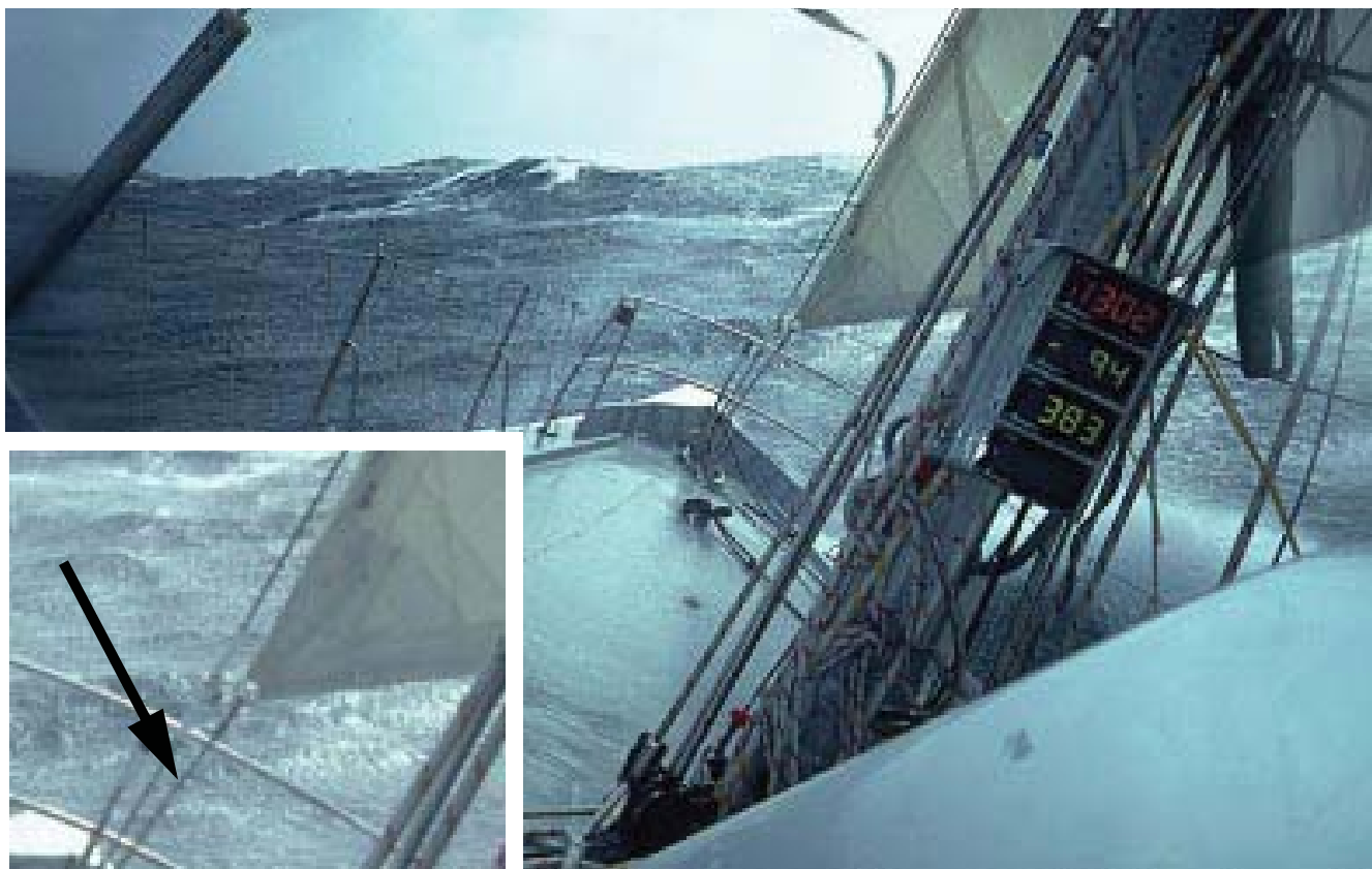
Fasizi deep in the Southern Ocean, broad reaching in 50 knots down a nice sea. The tack pennant (arrow and inset) keeps the sail well clear of the deck and any waves which wash aboard periodically.
