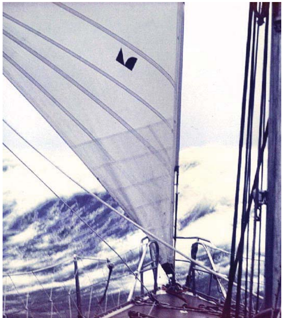
A high-clewed storm jib in the furious fifties aboard Ceramco New Zealand in the Whitbread Race. The clew is cut high so the sail will trim well off the wind as well as to windward. A high clew also keeps water out of the foot of the sail.
