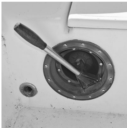
A diaphragm-type bilge pump mounted on the side of the cockpit that can be operated from the helm while underway.
