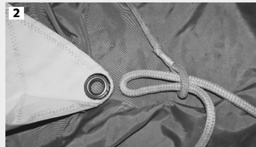
First, pass the middle of the sheet through the eye splice. It helps if the eye splice is sized for a snug fit.
