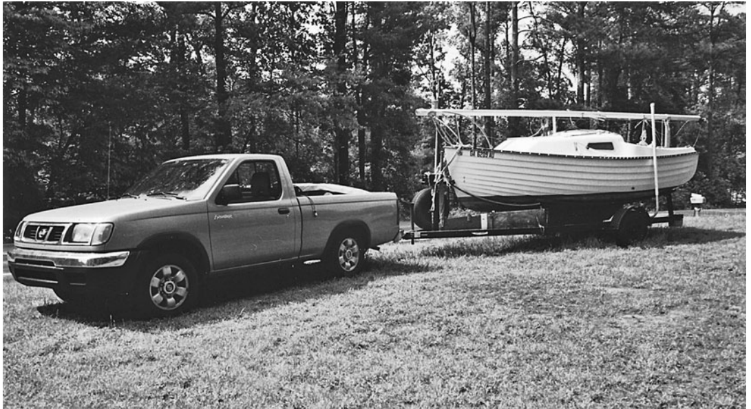
My Montgomery 17 on the day I purchased it. This trailer is a small float-on type, with PVC guide poles along the sides to help position the boat correctly when retrieving. Note that there's no transom strap in place, so I tied on a length of stout line for the trip and added attachment points later.
