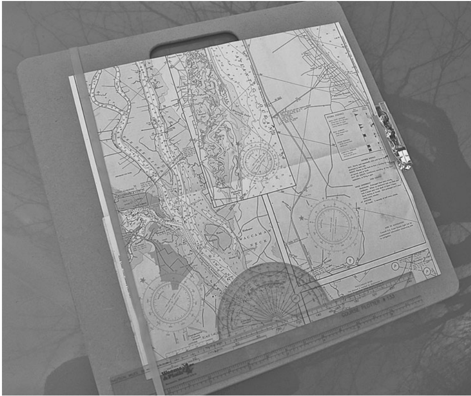
A sketch board used to hold a navigational chart.
