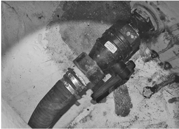
Seacocks should be double clamped, and a tapered plug (not shown here) should be located nearby.
