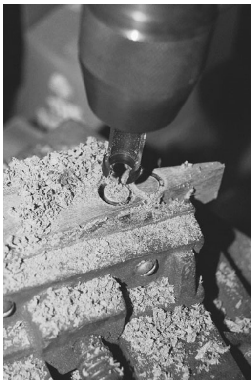
Step 7. Cut plugs to cover the mounting screws from a scrap of the same type of wood. Mount the rack on a bulkhead near your navigation area.
