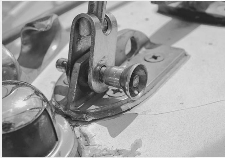
A ball-lock quick-pin—not to be used with standing rigging, but they can work well on a headsail track.
