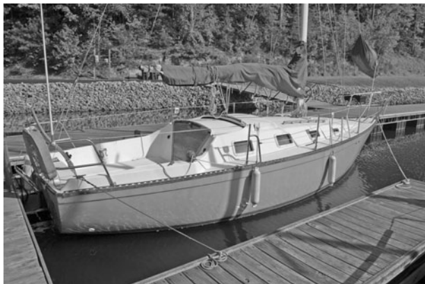
The Lancer 28: 28 feet long, 8-foot beam, 2-foot 10-inch draft; it displaces almost 5,000 pounds.
