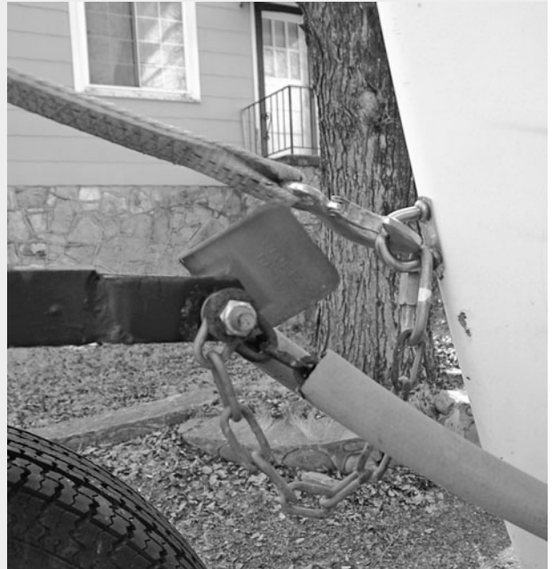
A safety cable on the bow eye.
