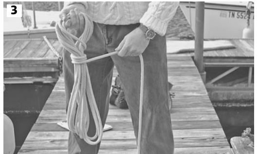
3 Take three or four turns around the entire bundle.
