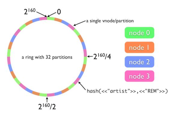
All nodes in a Riak cluster are equal. Each node is fully capable of serving any client request. This is possible due to the way Riak uses consistent hashing to distribute data around the cluster.
