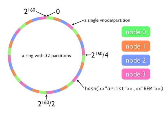
Nodes can be added and removed from the cluster dynamically and Riak will redistribute the data accordingly.
