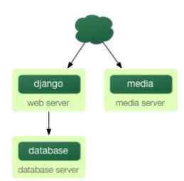
Ideally, this media server should run a stripped-down web server optimized for static media deliver. <u>lighttpd</u> and <u>tux</u> are both excellent choices here, but a heavily stripped down Apache could work, too.
