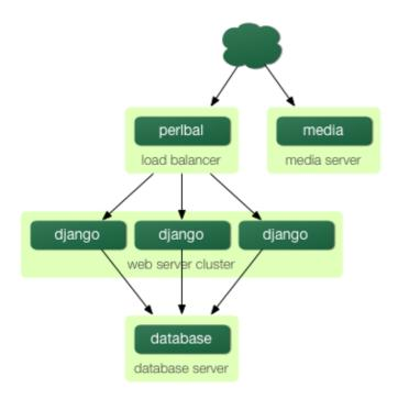
Notice that in the diagram the web servers are referred to as a "cluster" to indicate that the number of servers is basically variable; once you have a load balancer out front, you can easily add and remove backend web servers without a bit of downtime.
