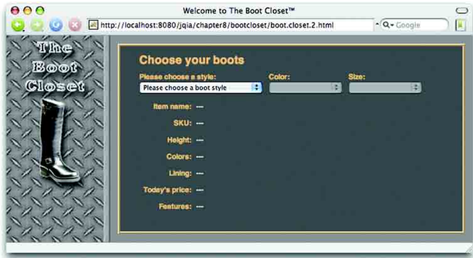
Figure 8.5 The initial state of the order form with the dependent dropdowns in an empty and disabled state
