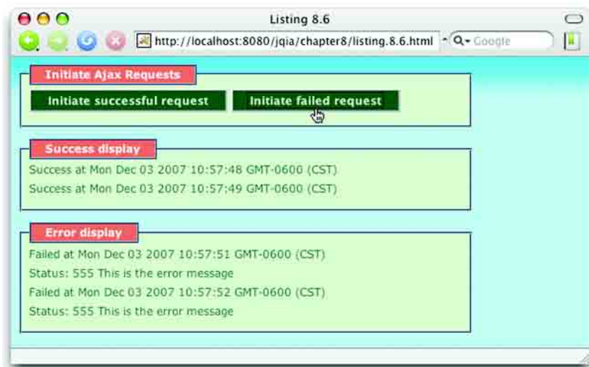
Figure 8.8 Clicking the buttons reveals how the callback functions get information and how they know which element they are attached to.
