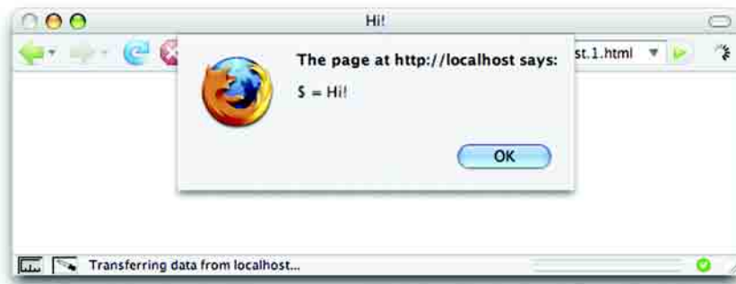
Figure 6.3 The $ says, “Hi!” as its redefinition takes effect within the ready handler.
