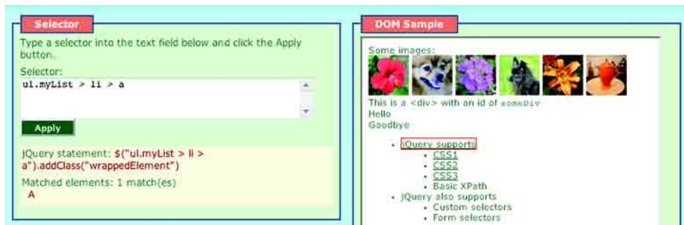
Figure 2.4 With the selector ul.myList > li > a , only the direct children of parent nodes are matched.
