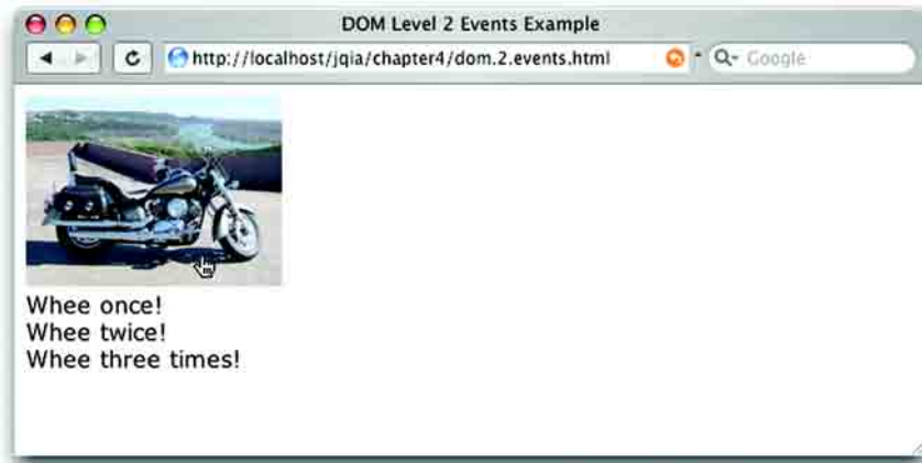
Figure 4.3 Clicking the image once demonstrates that all three handlers established for the click event are triggered.
