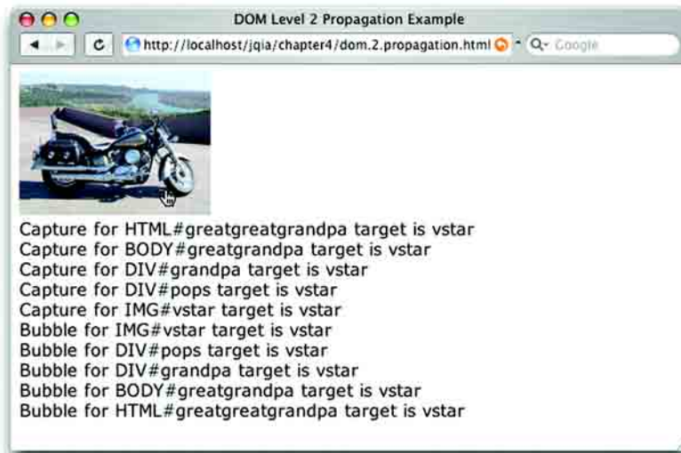
Figure 4.5 Clicking the image results in each handler emitting a console message that identifies the path of the event.
