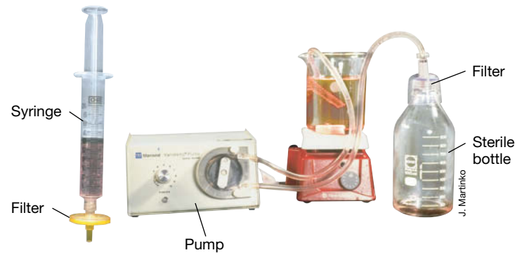
Figure 5.35 Membrane filters. Disposable, presterilized, and assembled membrane filter units. Left: a filter system designed for small volumes forced through the filter by a syringe. Right: a system employing a peristaltic pump for filtering larger volumes.
