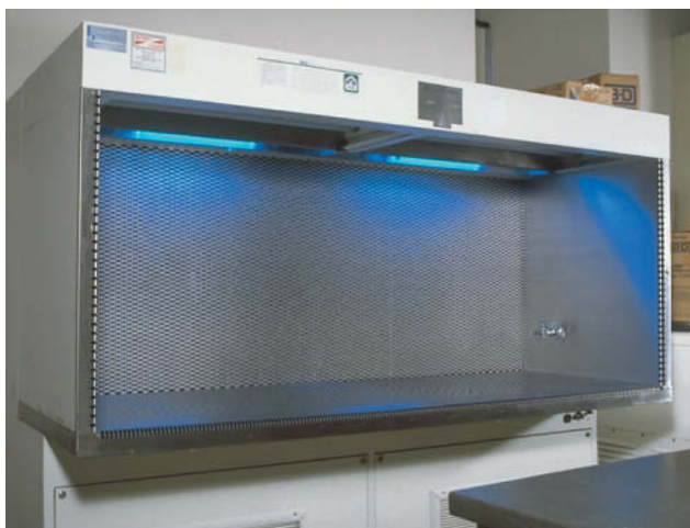
Figure 5.32 A laminar flow hood. An ultraviolet light source prevents contamination of the hood when it is not in use. When the hood is in use, air is drawn into the cabinet through a HEPA filter. The filtered air inside the cabinet is exhausted out of the cabinet, preventing contamination of the inside of the hood. The cabinet provides a contaminant-free workspace for microbial and tissue culture manipulations.
