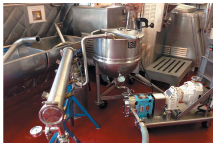
Figure 12.28 Application of CinderBio hyperstable enzymes for the cleaning of creamery equipment. These heat-stable enzymes clean industrial food-processing equipment as well as or better than traditional cleaning methods and do not generate large amounts of toxic wastewater.
