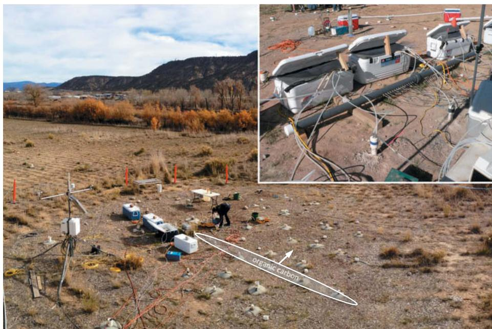
**Figure 22.6** Uranium bioremediation. An experimental plot at a United States Department of Energy uranium-contaminated site. Organic carbon (acetate) is being infused into the site (see inset photo) and travels in groundwater in the direction of the arrow shown in the main photo. Acetate is an electron donor for reduction of  $\text{U}^{6+}$  to  $\text{U}^{4+}$ , which immobilizes the uranium.
