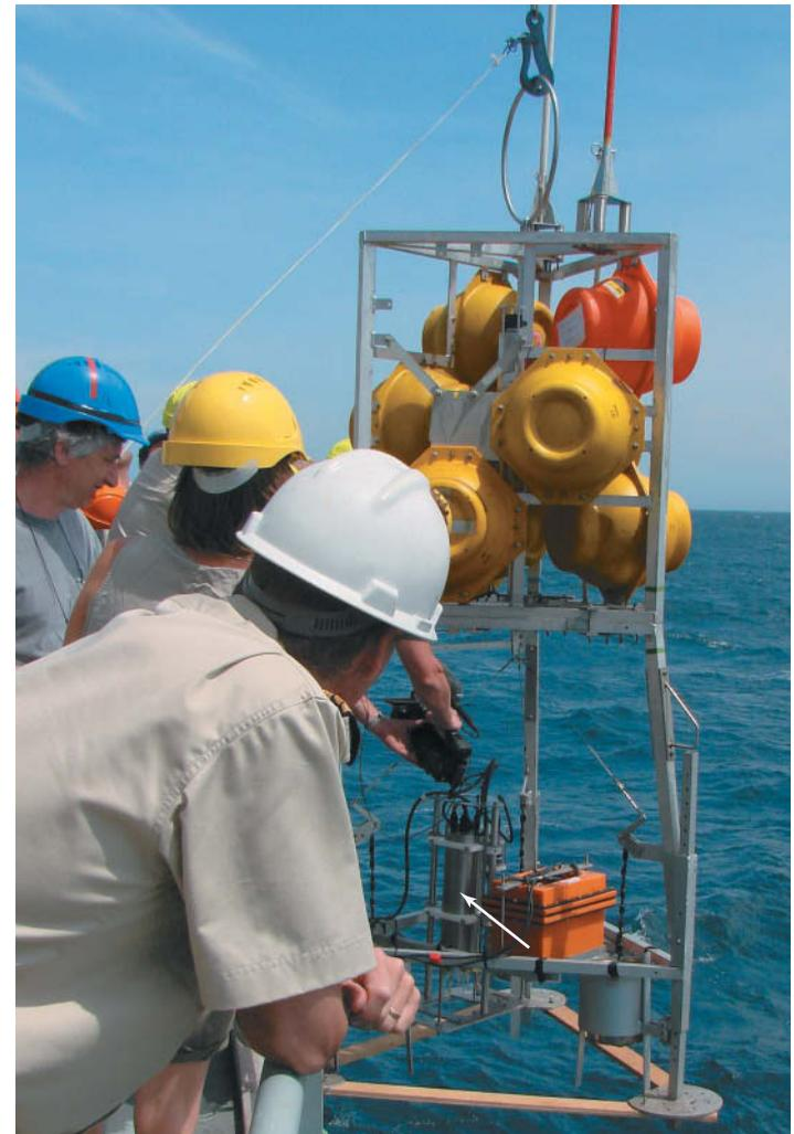
**Figure 19.28 Deployment of a deep-sea lander.** The lander is equipped with a bank of microsensors (arrow) to measure distribution of chemicals in marine sediments.
