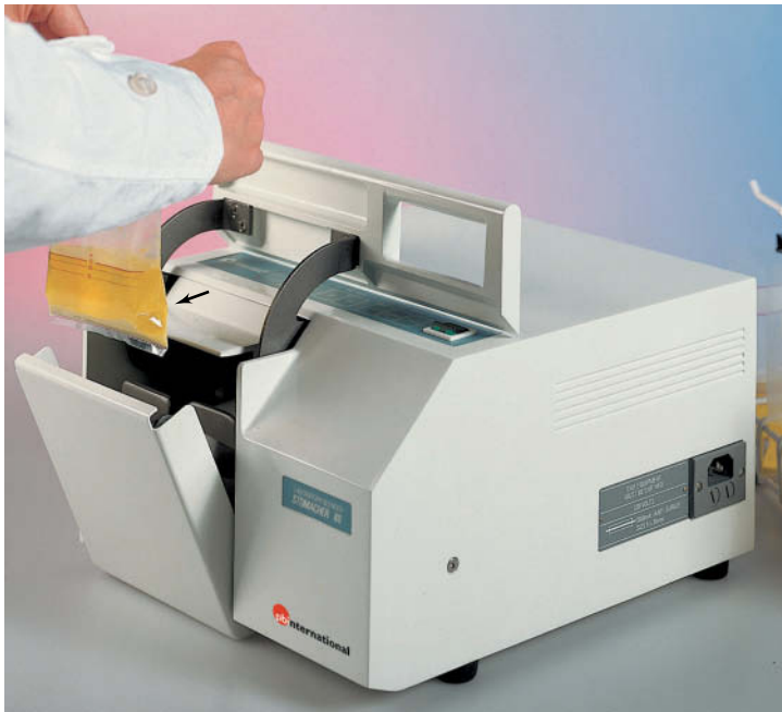
Figure 32.9 A stomacher. Paddles in this specialized blender homogenize the food sample contained in a sealed and sterile bag (arrow). The sample is first suspended in a sterile solution to form a uniform mixture.
