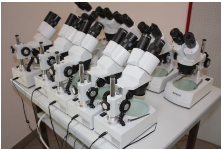
These stereo microscopes can be operated with a battery, thus making them independent from a power supply in a classroom.
