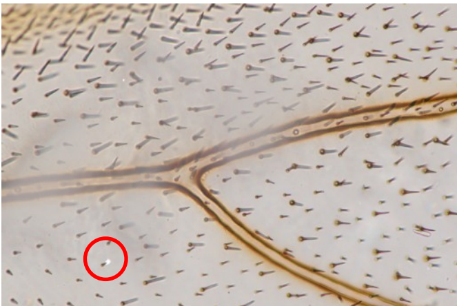
Despite the large amount of dust, the software was able to completely remove the disturbance. Notice that there are now brighter areas where the dust was located, as well as bright spots (circled). Fine-tuning the subtraction factor may help to reduce these bright areas.
