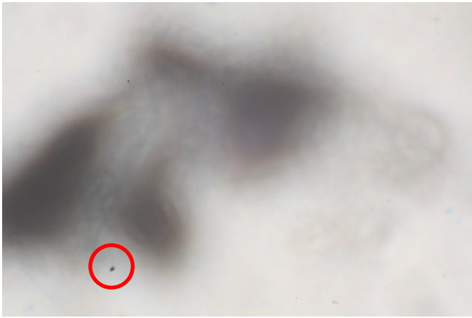
The background image. There is much dust in the optical system. For demonstration, I have placed an unrealistically large amount of dust on the microscope's lamp. The circle indicates dust which is missing on the micrograph to be improved (right).
