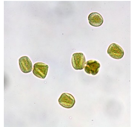
Euparal-mounted pollen. The Euparal brightened the pollen, but caused shrinkage.
