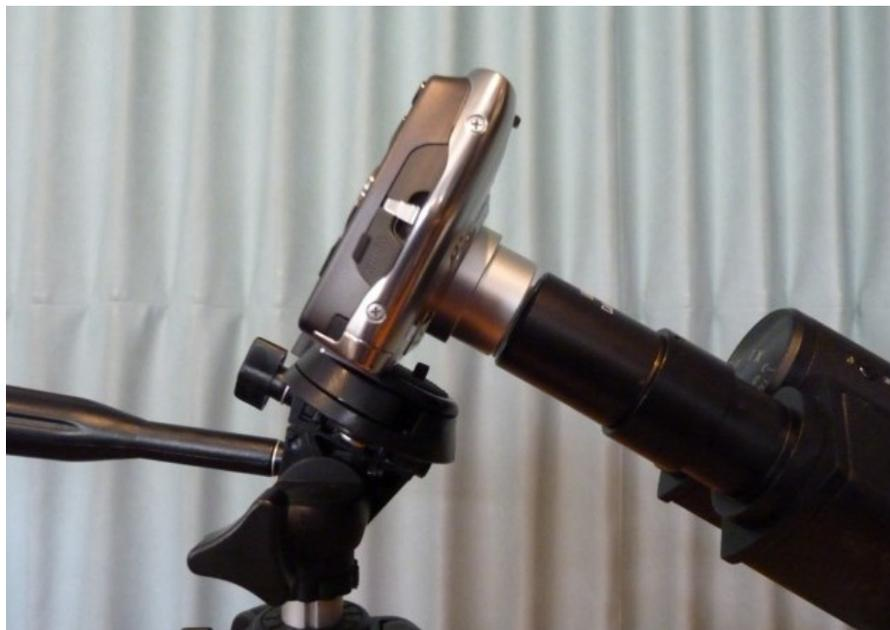
The camera to eyepiece distance depends on the eye relief of the eyepiece. Longer eye-relief eyepieces need a larger distance. An incorrect distance can cause vignetting.
