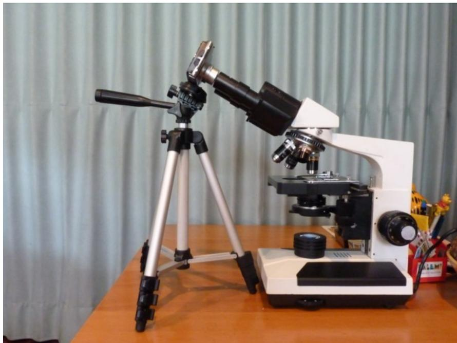
The complete set-up. The tripod is adjusted so that the camera's optics can be fully extended. The camera has to be in line with the eyepiece.
