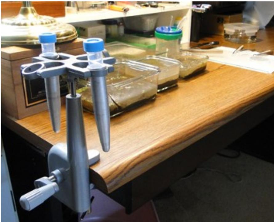
The hand centrifuge can be clamped to a table. Running the centrifuge requires sufficient space. You need space for operating the crank and for the rotating tubes, which swing into a horizontal position. Make sure that both tubes have the same mass, otherwise the system may start to vibrate. This also increases the wear on the gearing system and may possibly also un-rattle the whole system from the table.
