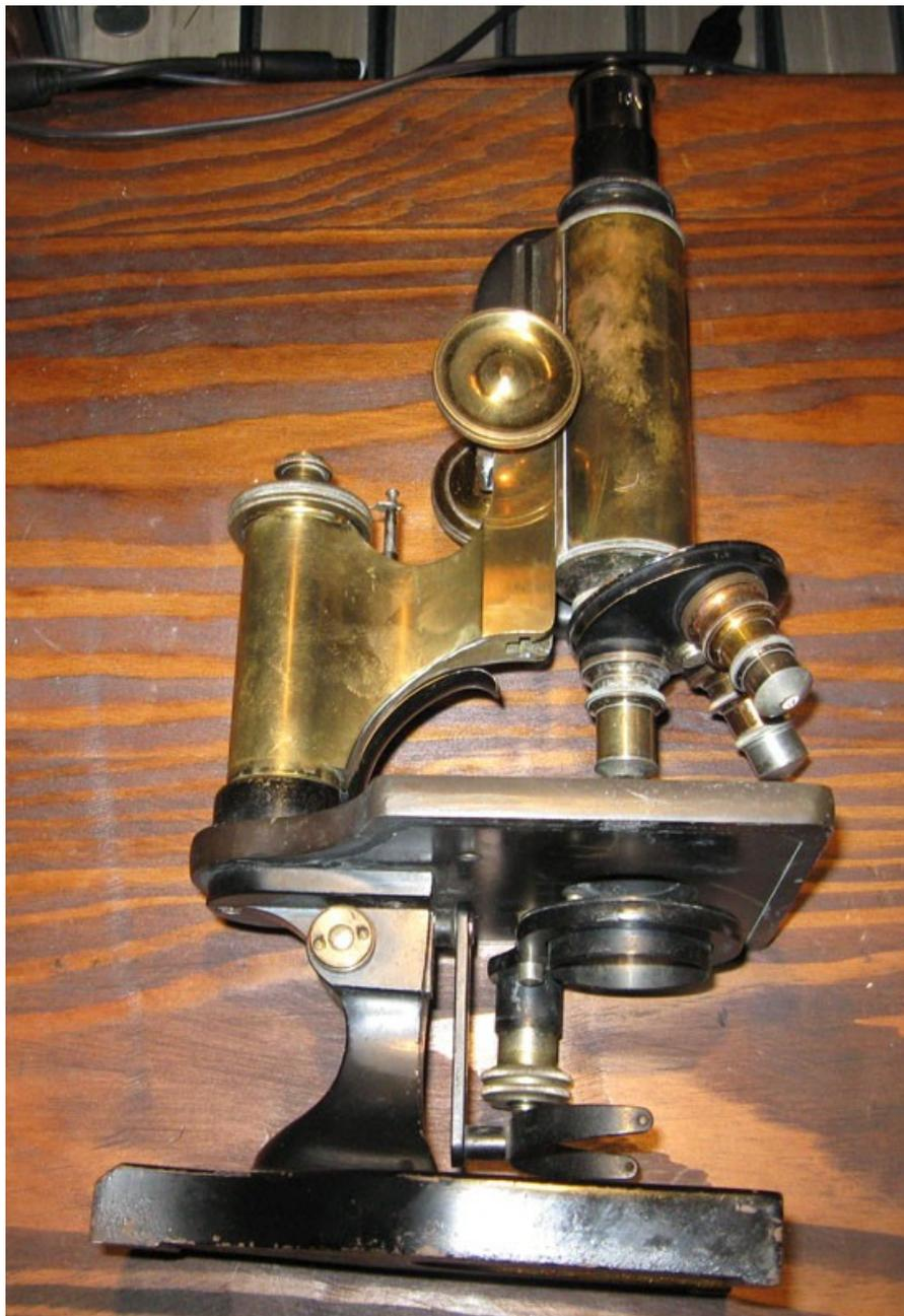
Fig. 2 - Behind curtain number two we have a circa 1912 Spencer Lens Co. stand. Has mirror fork and condenser holder but no mirror or condenser, coarse focus pinion axle slightly bent and the arm to stage connection is loose. This is close to the all brass style I was originally interested in. I will be attempting to adapt a condenser and mirror to complete this scope. Total with shipping \$57.00.
