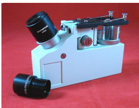
Figure 9 - Clone with Original Eyepiece Removed and Other Manufacturer's Eyepiece in its Place
