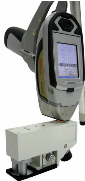
Figure 7 - Chemical Analysis of Clone Body Using X-Ray Fluorescence Spectrometer
