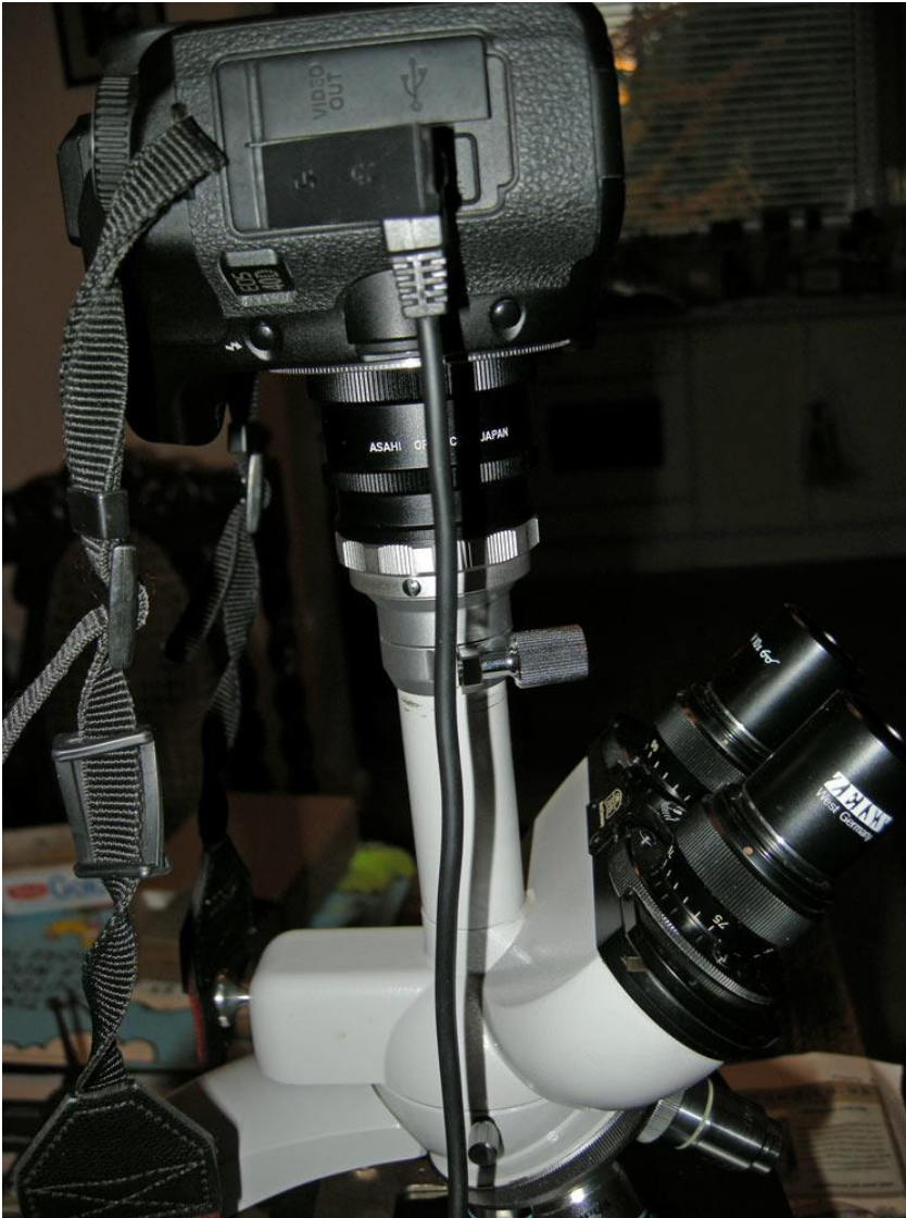
Canon EOS 40D camera mounted in a Zeiss Standard trinocular microscope with a Pentax adapter
