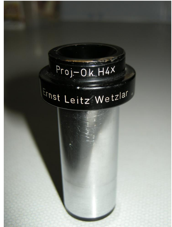
Leitz X4 compensating projection eyepiece
