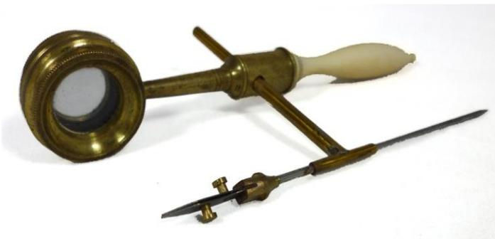
Figure 6. The "flower microscope", a fixed version descended from the original compass microscopes
