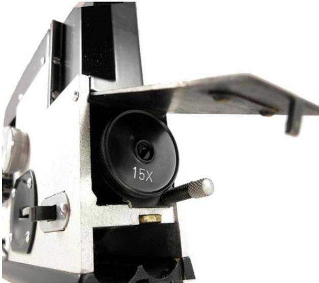
Figure 21. Hidden eyepiece and battery storage compartment
