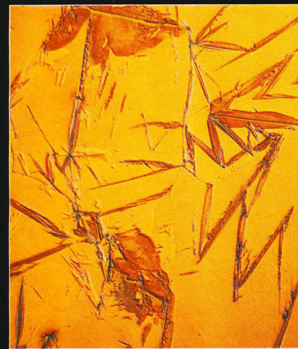
Martensite in Austenite 150 Cr6 Hardened in highly overheated state. Nomarski Differential Interference Contrast. Instrument: Zeiss AXIOMAT (upright version) Objective: Epiplanachromat 50x 0.95 HD Pol Magnification on film: 500x • Agfachrome 50 L 10x12 Preparation and photography: G. Wilpert, Carl Zeiss, Inc.
