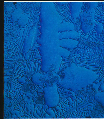
Steel hardened in highly overheated state. Nomarski Differential Interference Contrast. Instrument: Zeiss AXIOMAT (upright version) Objective: Epiplanachromat 100x 1.30 Oil HD Pol Magnification on film: 1000x • Agfachrome 50 L 4x5" Specimen preparation and photography: G. Wilpert, Carl Zeiss, Oberkochen
