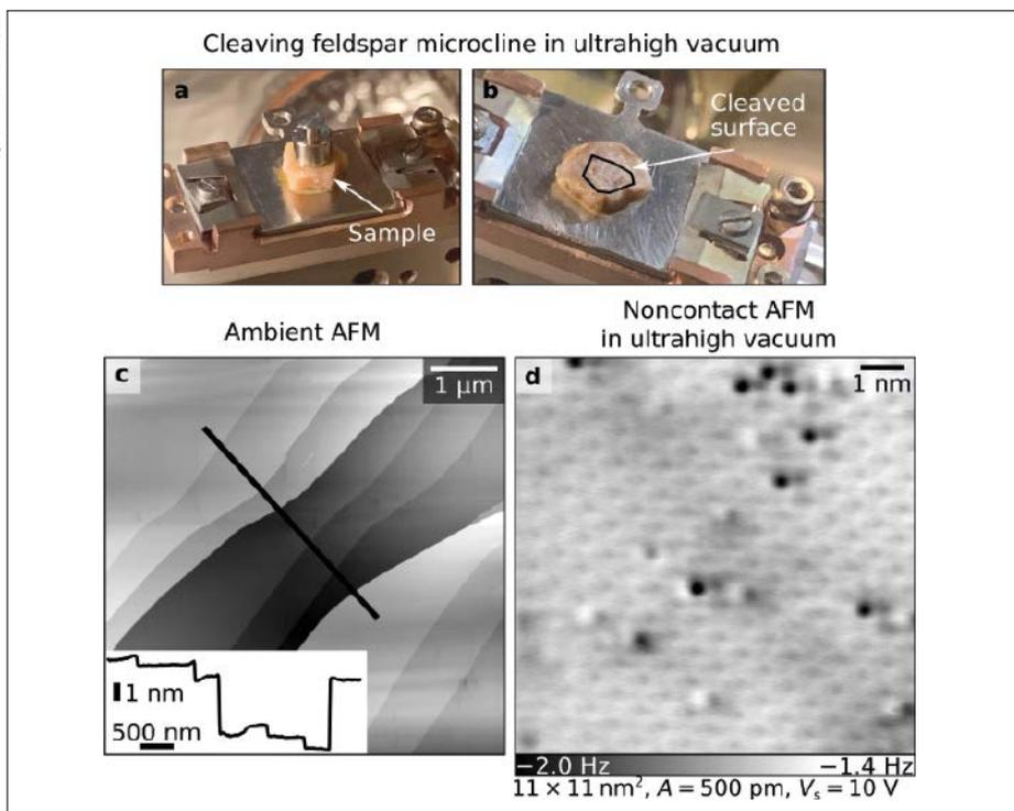
**Fig. 1:** (a, b) Cleavage of microcline feldspar in ultrahigh vacuum (UHV). A metal stud glued to the sample (a) is removed by applying a tangential force with a wobble stick (b). The resulting surface is atomically flat and clean and can be imaged with atomic resolution. (c, d) Surface morphology of cleaved microcline feldspar in ambient and non-contact UHV AFM. Point defects are visible on an otherwise atomically clean and periodic lattice. Adapted from ref. [3].
