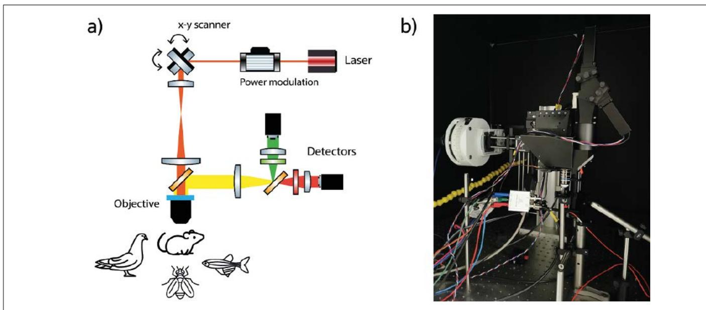
Fig. 2: a) A typical multi-photon microscope has a simple beam path. Light coming from femtosecond laser is scanned across the field of view of the objective lens. A non-descanned detection path collects as many non-ballistic emitted photons from the sample as possible. b) The simplicity of the beam path allows a wide range of *in vivo* studies such as at the Max-Planck Institute for Biological Intelligence.
