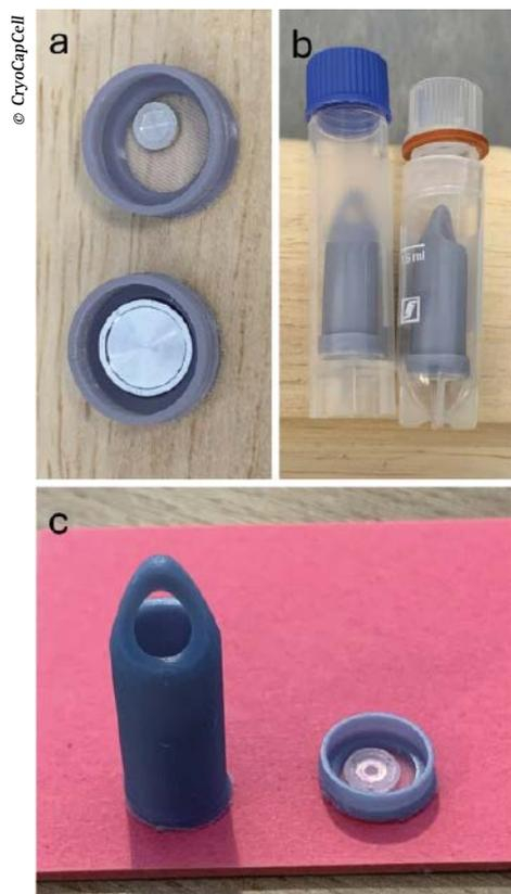
**Fig. 1:** The original version of the FS-basket. *a)* The lower part of the FS-basket with 3 mm (upper) and 6 mm (lower) carriers. *b)* Closed FS-baskets in cryo-tubes. *c)* The upper (left) and lower (right) part of the FS-basket with the Cryocapsule.
