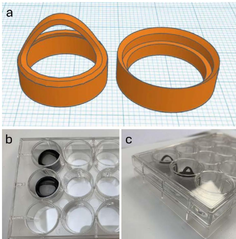
**Fig. 2:** The expanded version of the FS-basket. *a)* The schematic diagram of the new version of the FS-basket. *b)* The overview of the FS-baskets in a 12 well plate. *c)* The sideview of the FS-baskets in a 12 well plate.
