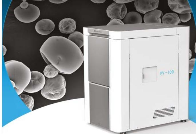
The PV-100 tabletop SEM from ModuleSci offers exceptional resolution in a compact package. Featuring a 5-axis stage and PICOSMART software, the PV series is the ideal solution when lab space is at a premium.
