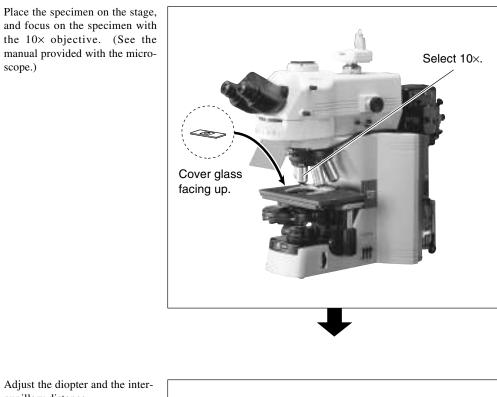
5 Adjust the diopter and the interpupillary distance. (See the manual provided with the microscope.)
