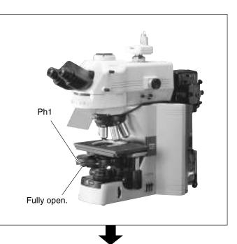
Center the Ph annular diaphragm. This adjustment is very important. Do not skip this step. (p. 23)
