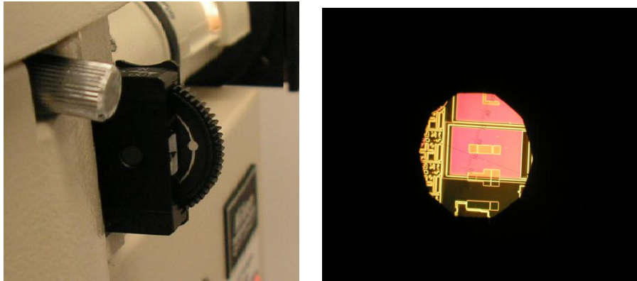
Rotate polarizing wheel: until ● coincidence with ► to use polarizer filter
