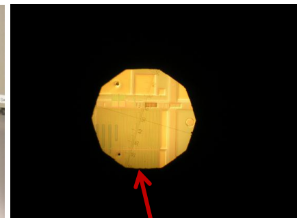
Aperture diaphragm (N.A. diaphragm ) (○ → ●) Stopped down to 70-80% of NA. OBJECTIVE
