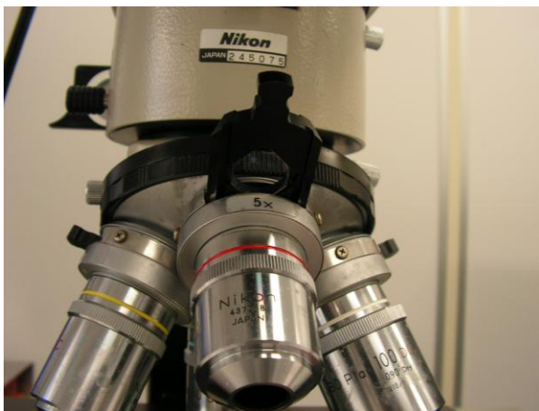
Polarizer push IN is out of optical path
