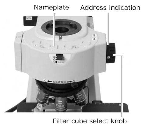
For clarity, the eyepiece tube is not shown here.
