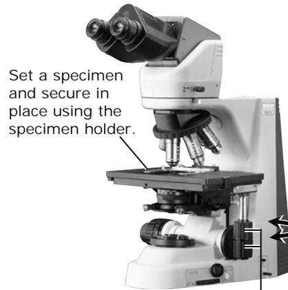
Move the portion to be viewed into the optical path using the XY stage knobs.
