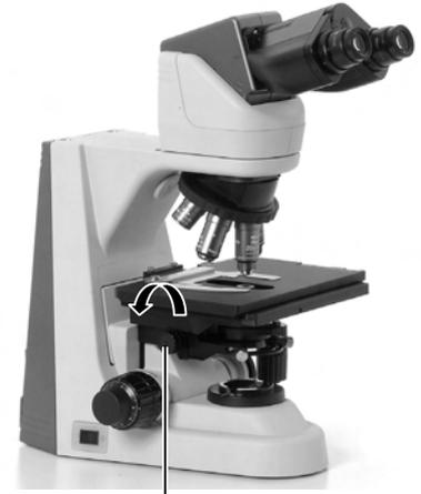
Raise the condenser using the condenser focus knob.
