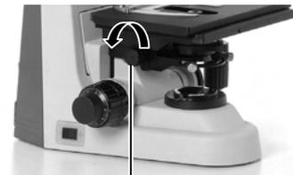
Raise the condenser using the condenser focus knob.
