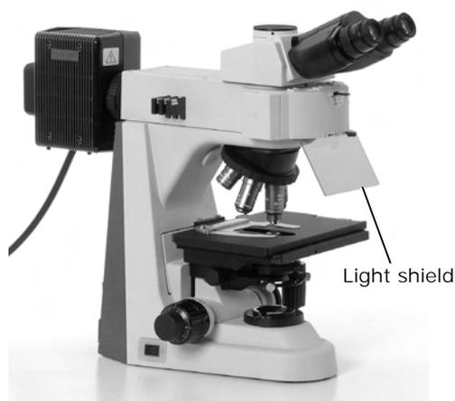
Light shield fitted in place
