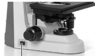
Press the power switch to the "O" position.
