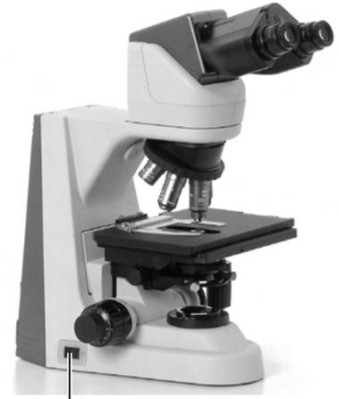
Press the power switch to the "I" position.
