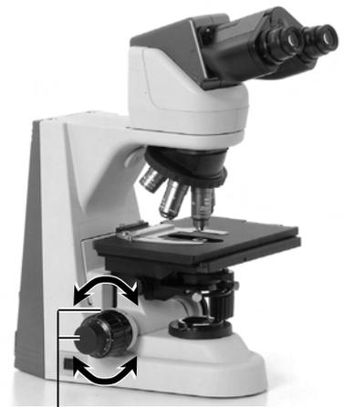
Focus on the specimen using the coarse and fine focus knobs.
