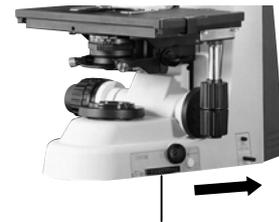
Turn the field diaphragm knob and stop down the field diaphragm to its minimum setting.
