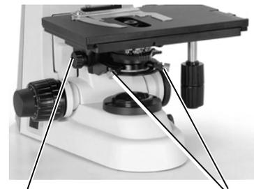
Condenser focus knob      Condenser centering screws
