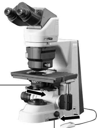
Fully open the aperture diaphragm using the aperture diaphragm knob.
