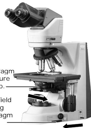
Fully open the aperture diaphragm using the aperture diaphragm knob.
