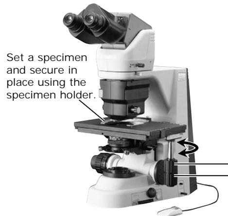
Move the portion to be viewed into the optical path using the XY stage knobs.
