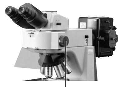
Select a cube using the filter cube switching knob.
