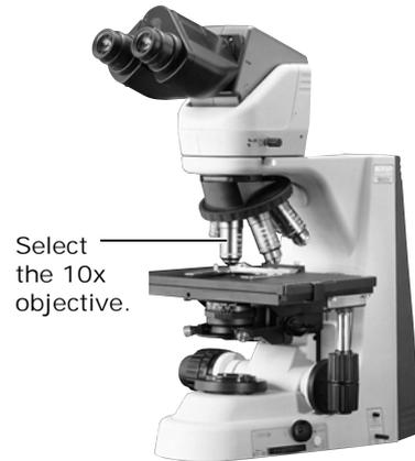
**5 Set a specimen and move the portion to be viewed into the optical path.**
