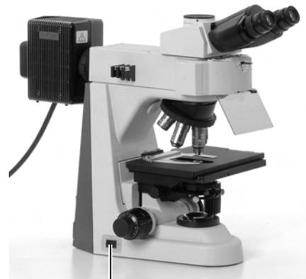
Press the power switch to the "O" position.
