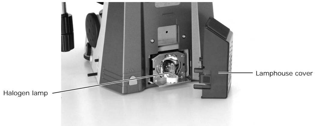
1.2 Names of Parts Used to Make Adjustments
