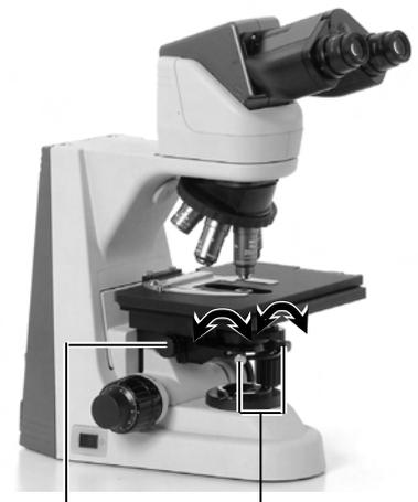
Focus the condenser using the condenser focus knob.
