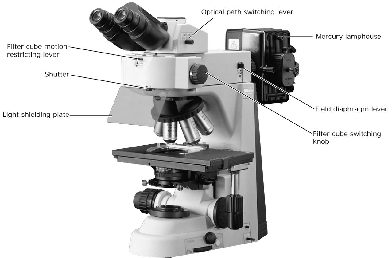
(Mercury lamps require a separate power source.)
