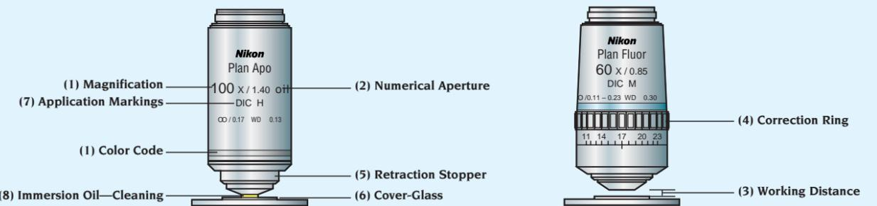
Nikon offers a wide variety of CFI objectives. To assist the user they are clearly marked with information on the objective barrel such as: which DIC module or Phase Ring to use.
