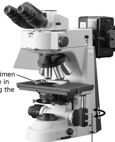
Set a specimen and secure in place using the specimen holder.
