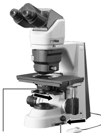
Fully open the aperture diaphragm using the aperture diaphragm knob.
