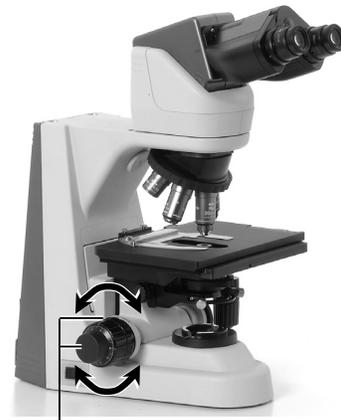
Focus on the specimen using the coarse and fine focus knobs.
