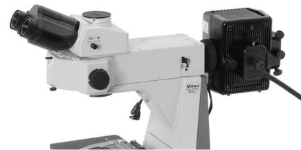
Mercury lamphouse attached in place
