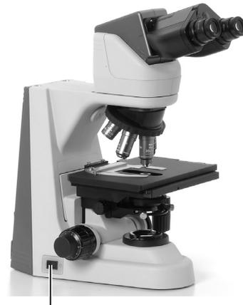
Press the power switch to the "I" position.
