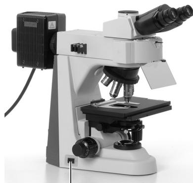
Press the power switch to the "O" position.
