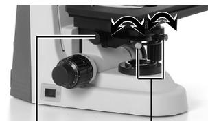
Focus the condenser using the condenser focus knob.
