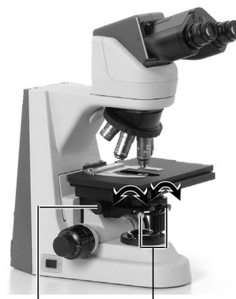
Focus the condenser using the condenser focus knob.
