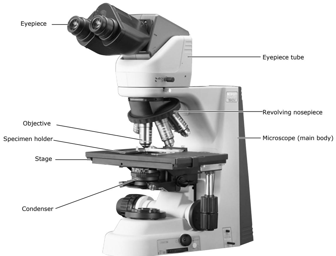
**1.2 Names of Parts Used to Make Adjustments**
