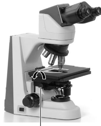
Raise the condenser using the condenser focus knob.
