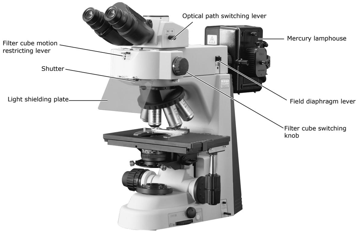
(Mercury lamp requires a separate mercury lamp power supply.)
