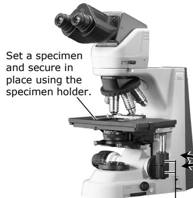
Move the portion to be viewed into the optical path using the XY stage knobs.
