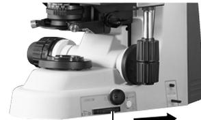
Turn the field diaphragm knob and stop down the field diaphragm to its minimum setting.
