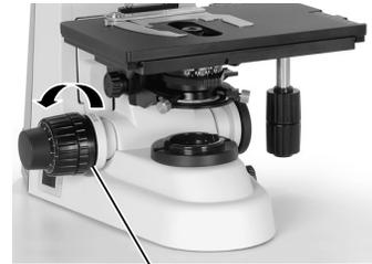
Coarse focus torque adjustment knob
