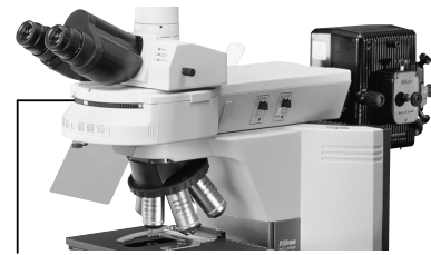
Rotate the excitation method switchover turret.
