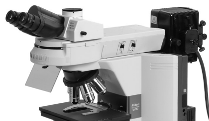
Light shield attached (with Epi-illumination attachment)
