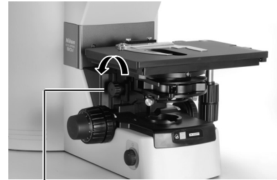
Raise the condenser using the condenser focus knob.
