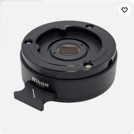
Nikon Microscope Intermediate Tube with Simple Analyzer Slider
