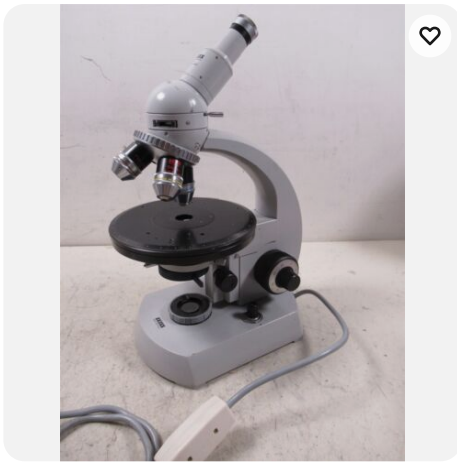
Zeiss Standard Polarizing Monocular Microscope w/ Bertrand Lens & Rotating Stage
