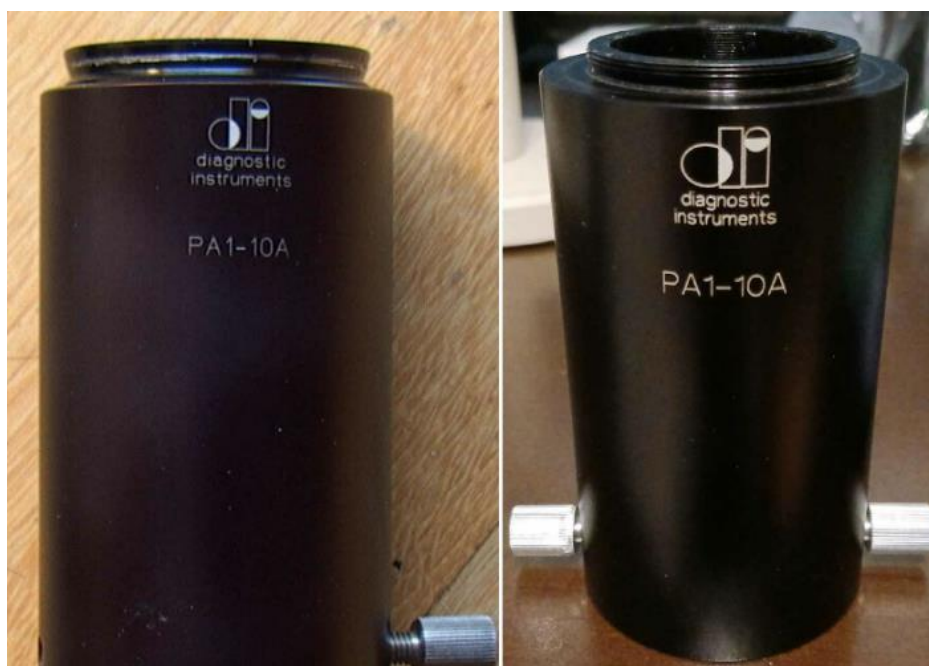
Diagnostic Instruments PA1-10A Adapters, female threads (left) and male threads (right, photo courtesy Joe Haralson)
