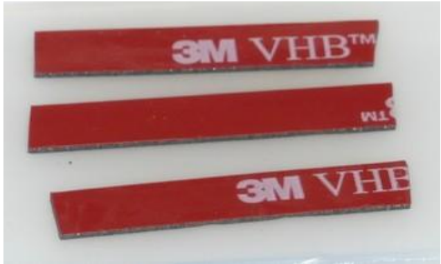
3M VHB Tape to secure wires.
