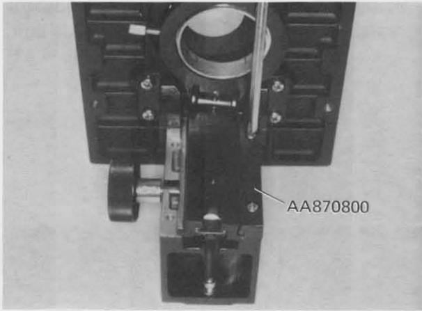
5-2 By removing two Screws CUK3x10SA, dismount right Dovetail AA870800. (See Fig. 5-2)
