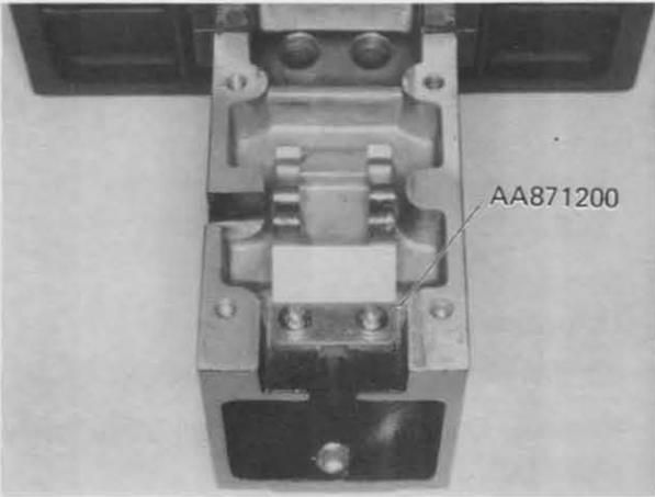
5-4-6 Dismount Pinion holder AA871200 by removing two Screws CUK3x5SA.
