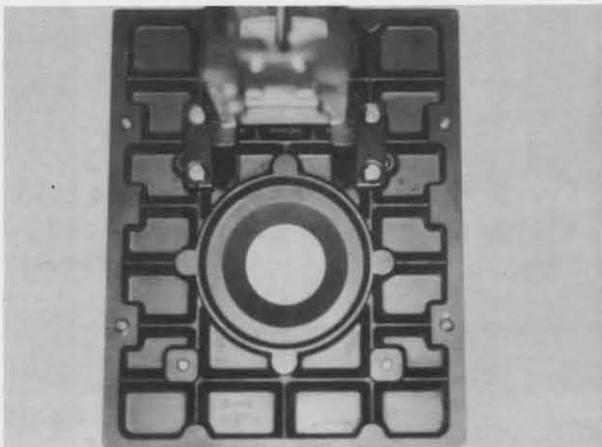
6-1 Reassemble Stage plate AA871800 with Block AA870500 by using four Screws CUK4x10SA.
