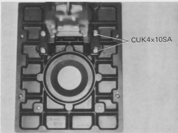
5-4-7 Detach Stage plate AA871800 by removing four Screws CUK4x10SA. (See Fig. 5-9)
