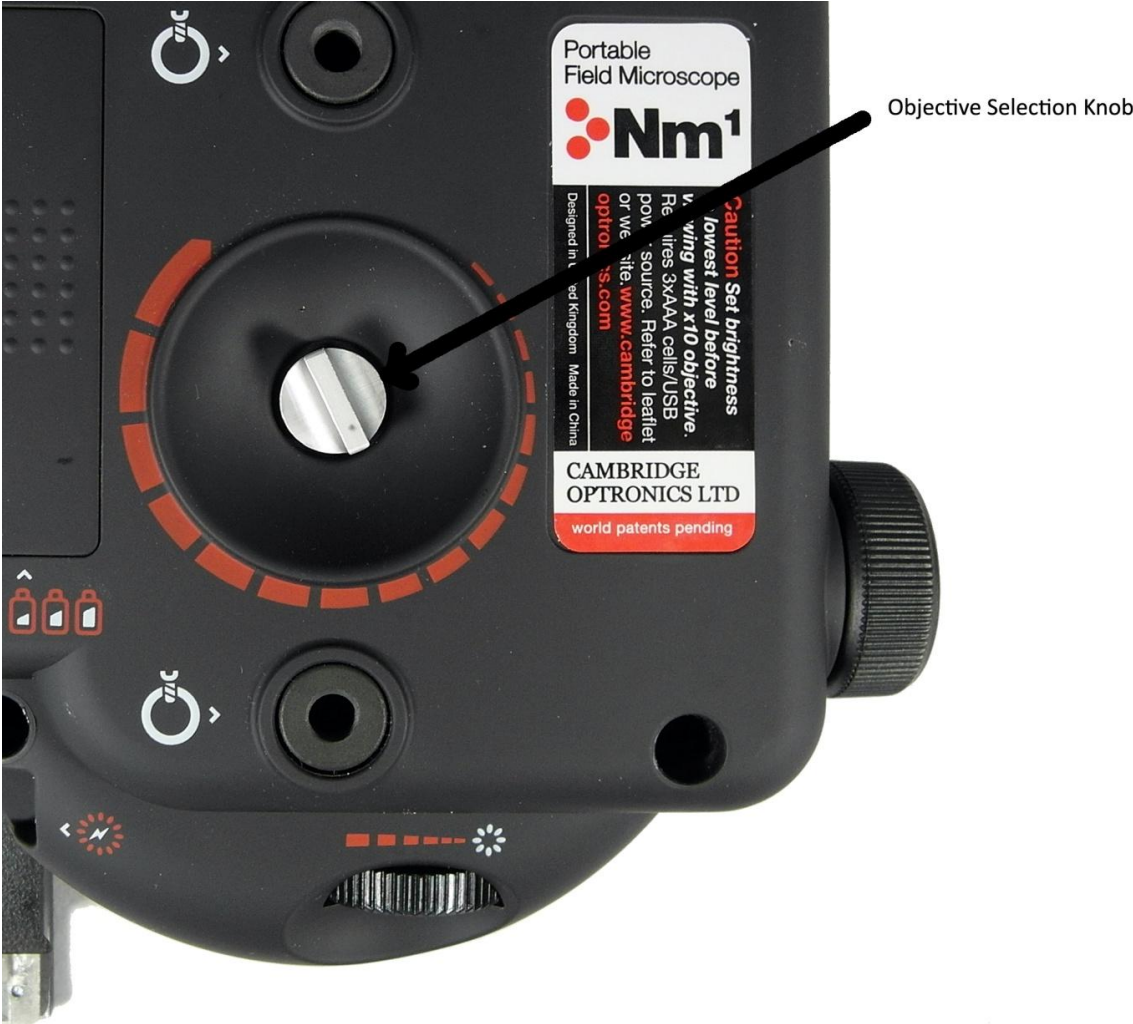
Figure 15. Rotating knob under the microscope, used to select objectives
