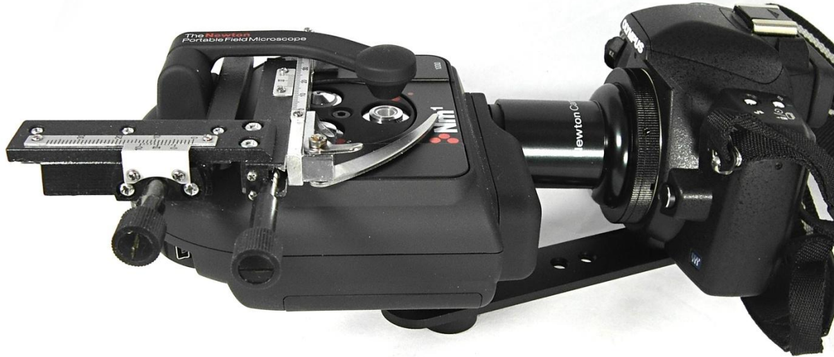
Figure 5. Olympus DSLR mounted to Newton Microscope
