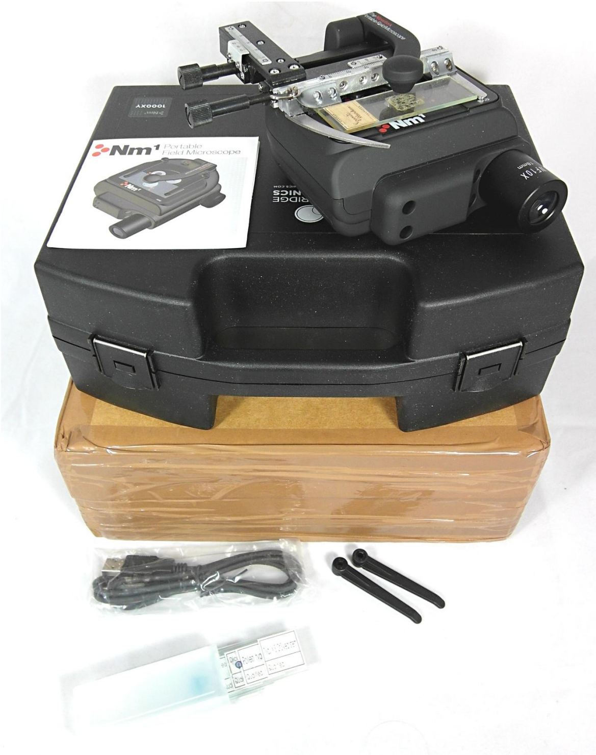
Figure 8. The Newton Microscope, case, and accessories outside of their shipping box. Slide on microscope is not included.
