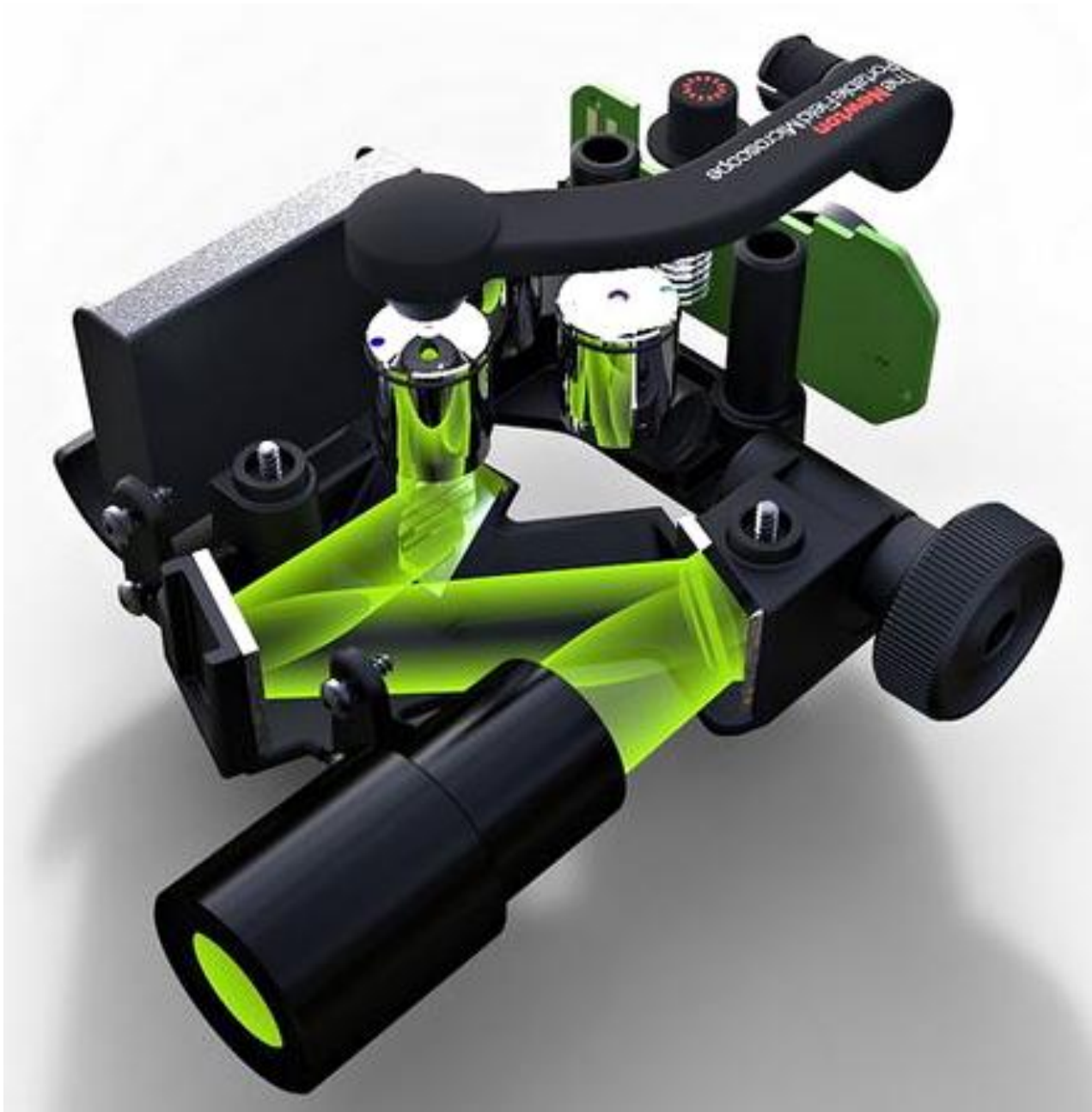
Figure 6. Newton Microscope optical path. Courtesy, and with permission, of Rick Dickinson
