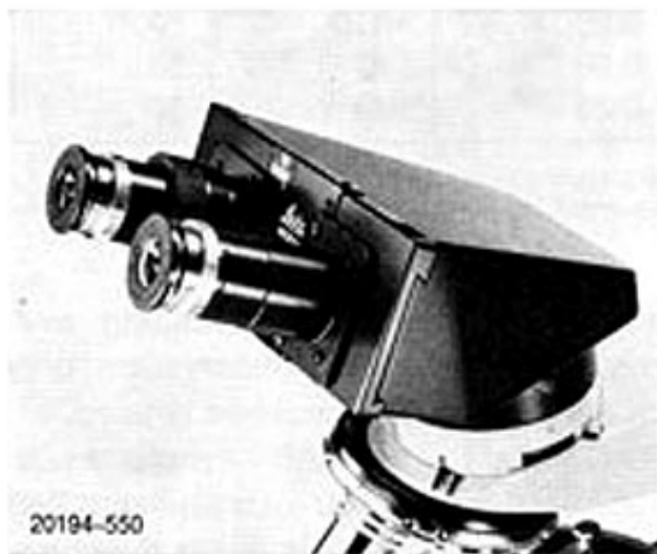
Fig. 5 Inclined binocular pol tube S 20 For orthoscopic observation. Conoscopy possible only with the pinhole stop, which is inserted in the eyepiece tube instead of the eyepiece.
