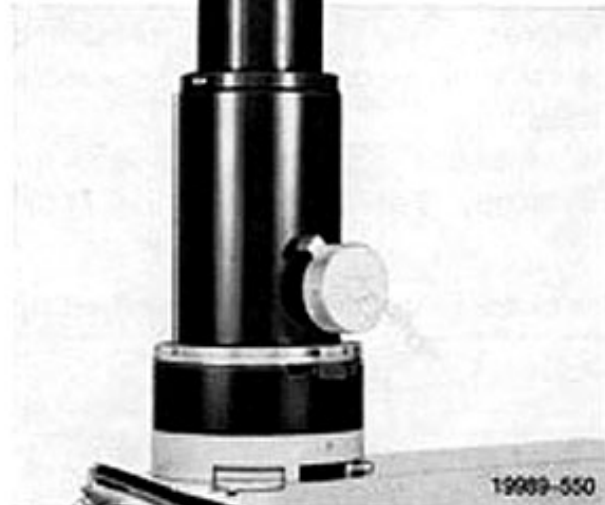
Fig. 4 Straight pol tube O 15 With disengageable Bertrand lens. Disengageable pinhole stop for conoscopy of small grains. Application: Wright eyepiece and micro-attachment for the LEICA®.
