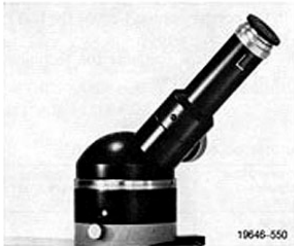
Fig. 3 Inclined monocular pol tube P 12 Standard equipment for monocular observation, fitted with disengageable Bertrand lens. Disengageable pinhole stop for conoscopy of small grains.
