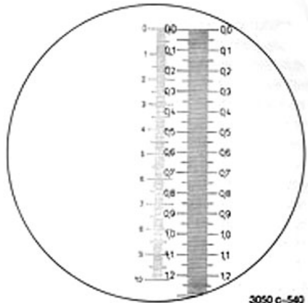
Fig. 17 Division of the graticule in the eyepiece and image of the stage micrometer
